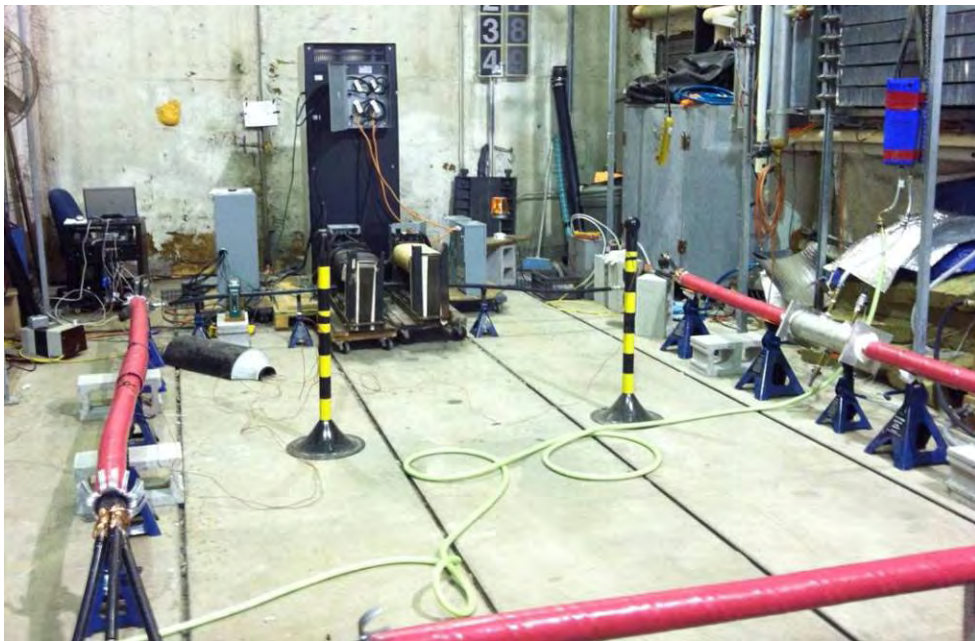
Figure 2.5: Water Penetration test setup
